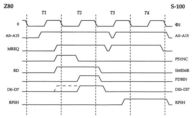
Not only are these data bus control signals important during I/O reads and writes; they actually arbitrate traffic to the Z80 data lines for all data reads and writes. While the S-100 bus has separate lines for data in or data out, the Z80 has 8 bidirectional data lines. PDBIN is used to route incoming bus data to the Z80, while PSYNC is used to route outgoing Z80 data to the bus.
