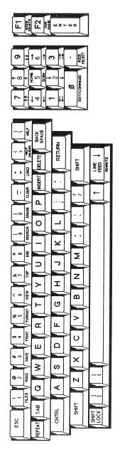
Figure 1. The complete Eagle keyboard. Note the labels on the *front* of many of the keys.
