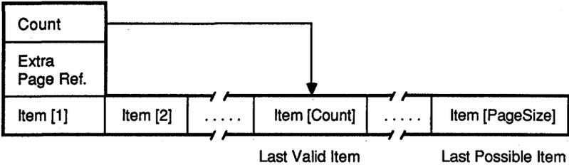
*Figure B-4. Structure of a Page in an Index File*
